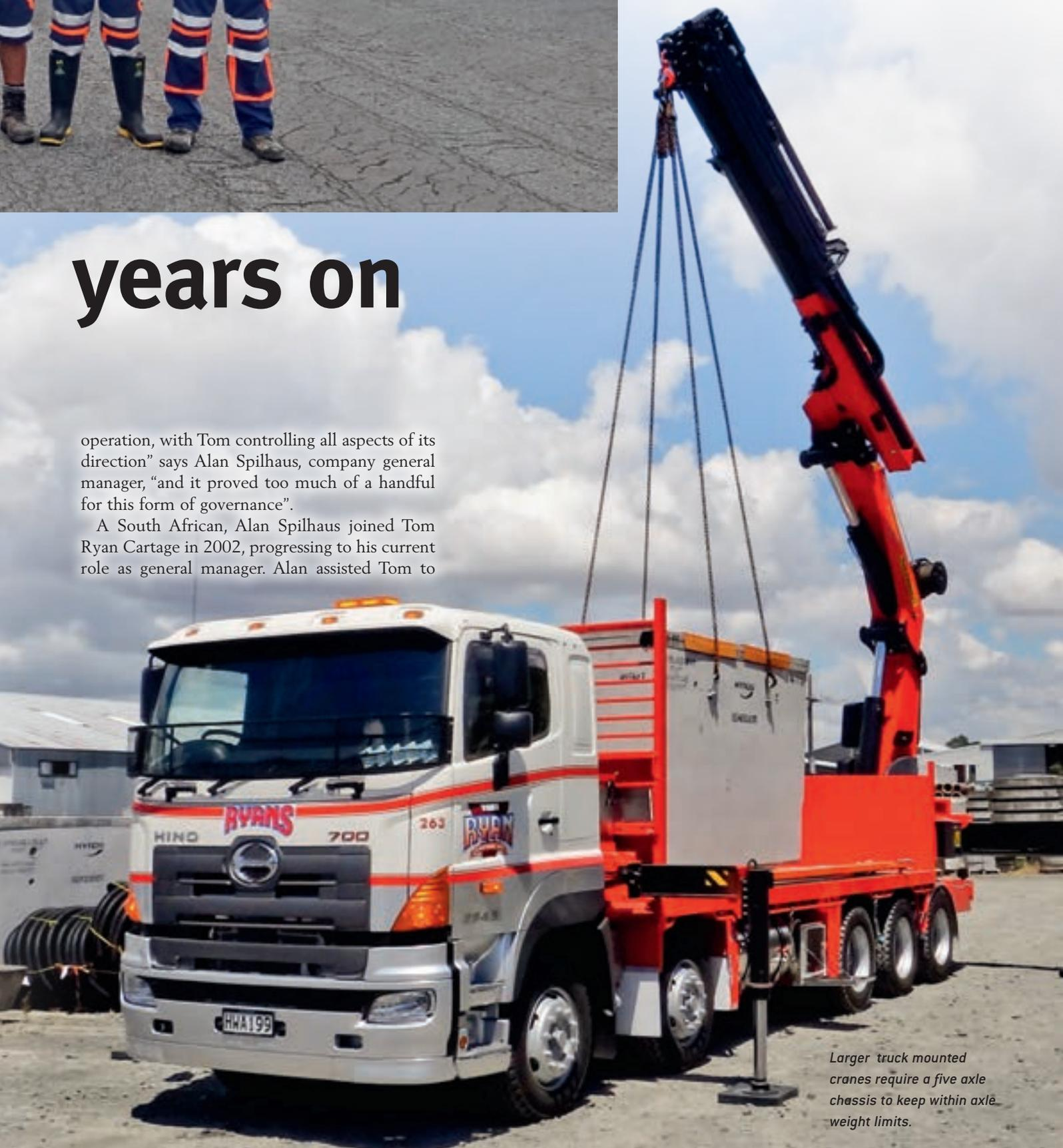
*Larger truck mounted cranes require a five axle chassis to keep within axle weight limits.*
