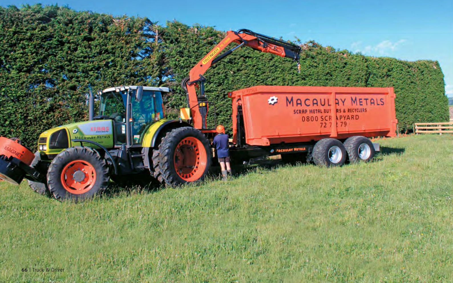
Below: This offroad hook-loading trailer was the ingenious answer to the problem of carting bins of electricity pylon scrap from inaccessible locations to highway bin trucks
