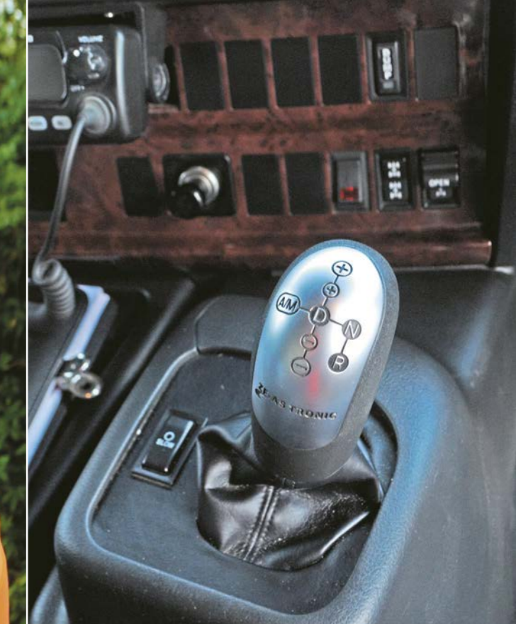
Right: Whether in manual or auto, the short gear selector makes the ZF AS Tronic Proshift 16 very simple to operate
