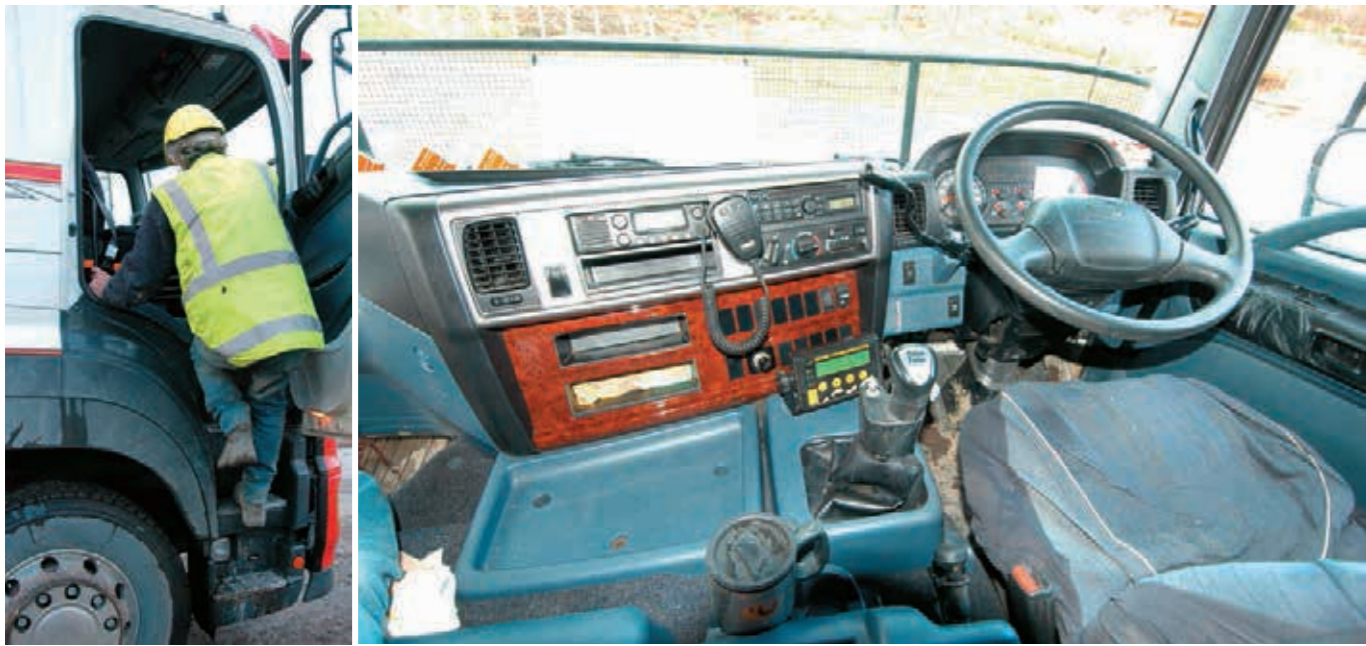
Above left: Getting in and out of the cab is easy, courtesy of good grabhandles and three non-slip, grated steps Above right & below right: Low-frills cab still has everything you need, says driver – including simple, easily-seen dash controls Below left: Checking the oil doesn't even require lifting the front inspection flap
