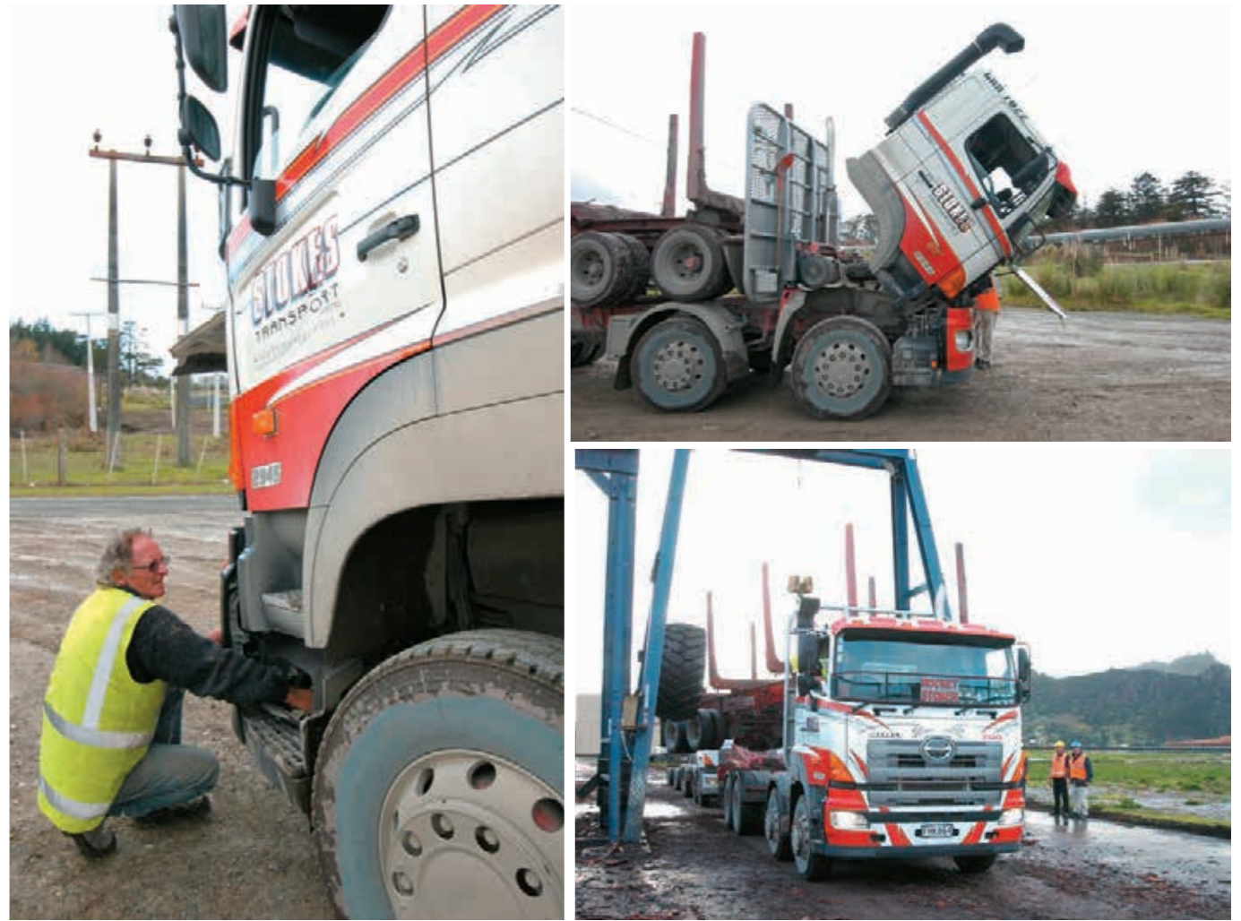
Above & top right: There's been no call for Gary to lift the cab before our test, so it takes a while to activate the electric/hydraulic lift Lower right: It's before 8.30am and, as the Patchell trailer is loaded onto the Hino for the trip back to the forest, Gary's already done a third of his day's work
