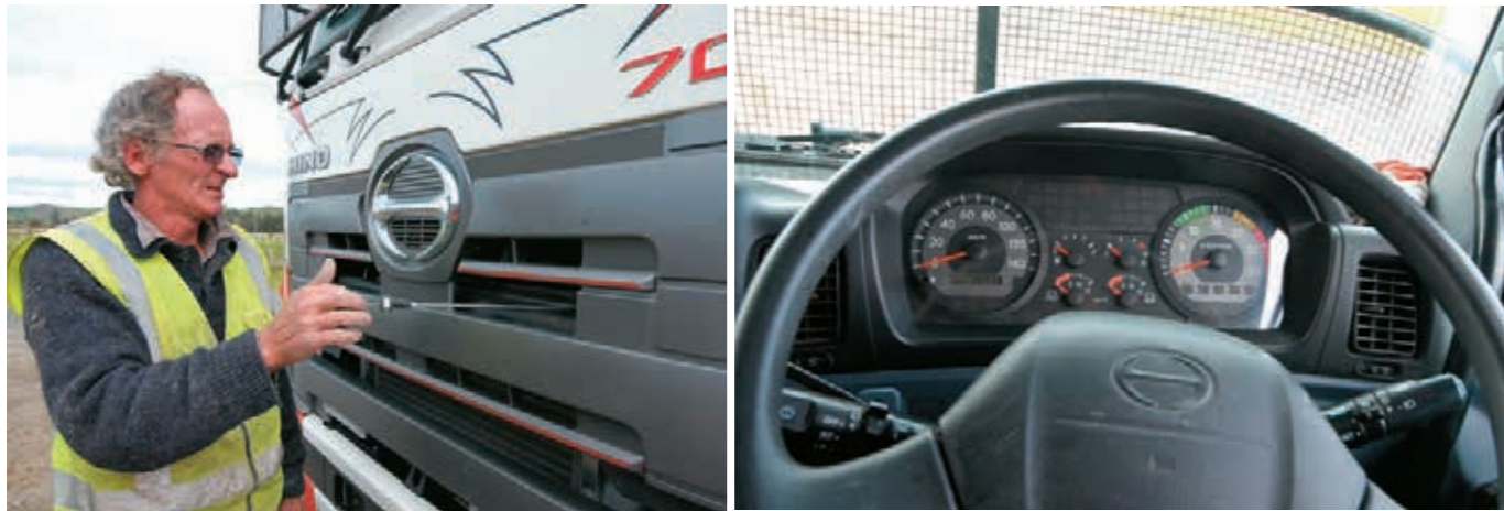
Above left: Getting in and out of the cab is easy, courtesy of good grabhandles and three non-slip, grated steps Above right & below right: Low-frills cab still has everything you need, says driver – including simple, easily-seen dash controls Below left: Checking the oil doesn't even require lifting the front inspection flap
